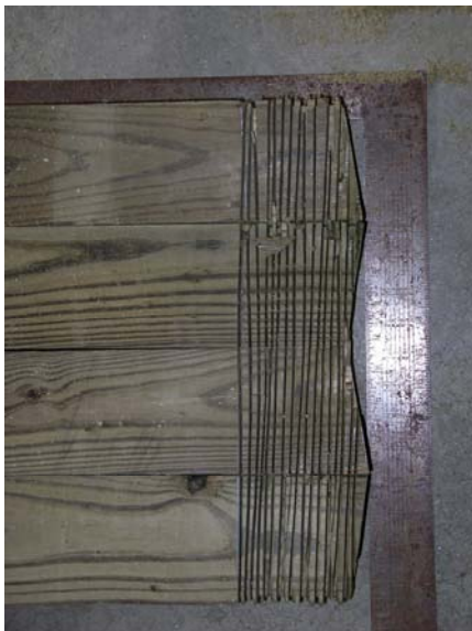
Photo 2-3: Alignment at top / grooves cut but not chiseled out. Clear the grooves with a wide chisel and a very coarse rasp.
